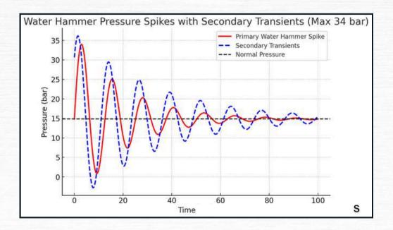
Here is a graph showing pressure spikes during a water hammer event. The red curve represents the sudden surge in pressure, followed by oscillations that gradually decay over time. The dashed black line represents the normal pipeline pressure.
