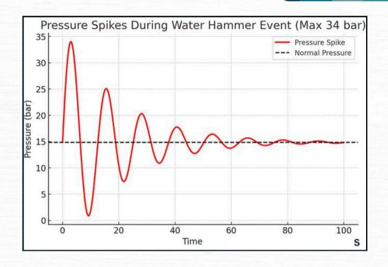
Here is a graph showing pressure spikes during a water hammer event. The red curve represents the sudden surge in pressure, followed by oscillations that gradually decay over time. The dashed black line represents the normal pipeline pressure.
